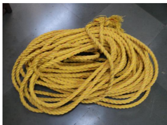
22 mm thick nylon rope for climbing trees
