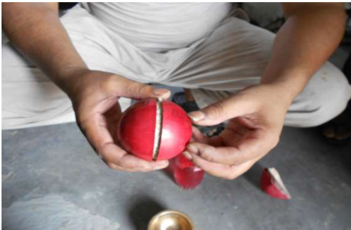
Cricket ball with leather outer case ready for stitching process
