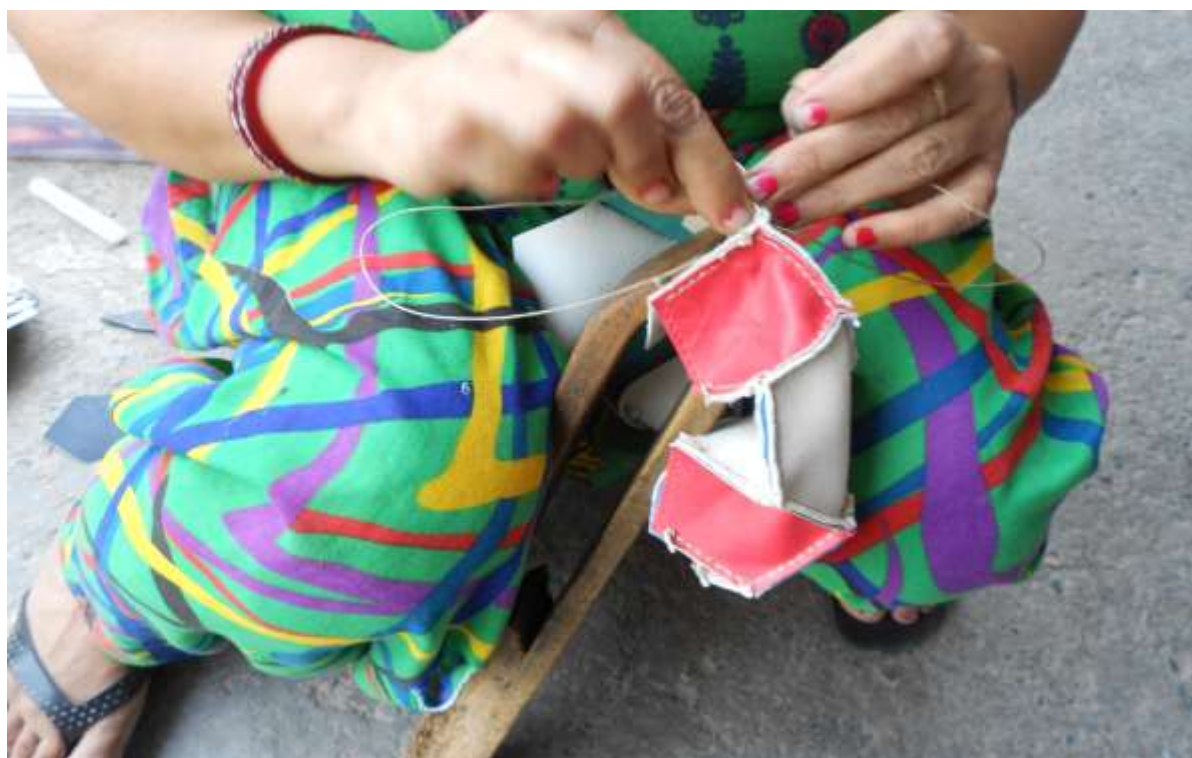
Woman at stitching of inflated ball at house– Non leather material used
